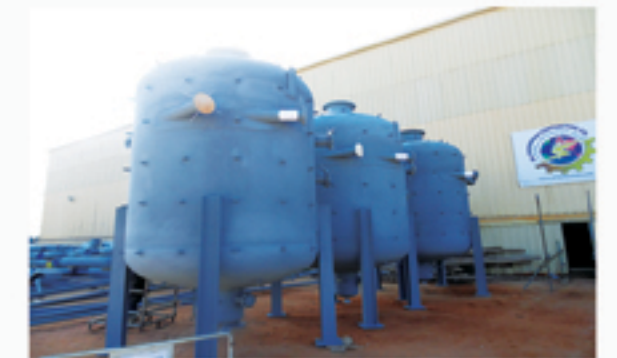
» Blowdown tank for West Damietta power station.
