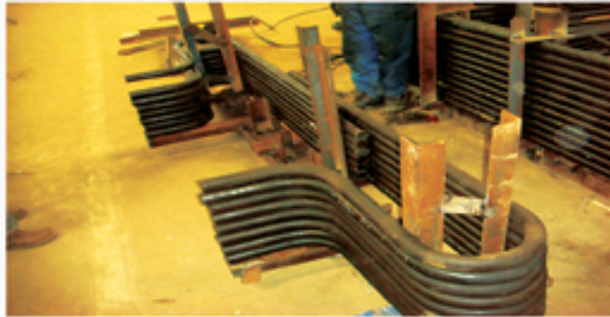
» Super heater coil element tube for Abu Qir thermal power station.
