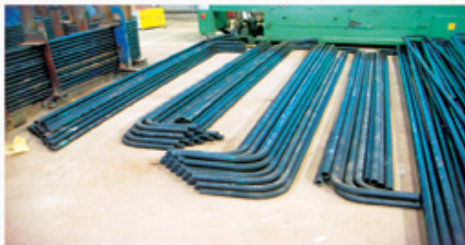
» Heat treatment for Super heater coil element tube for Abu Qir thermal power station.
