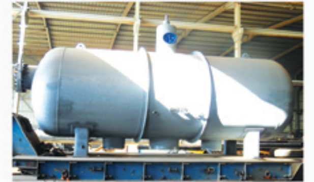
» Deaerator tower for El Shabab power station .
